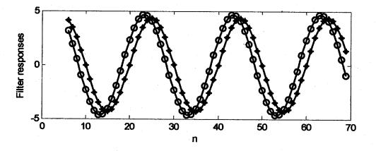
From this plot it is seen that the filter responses are similar, except that the response to the filter in Problem 1.14 is faster (by about 2 time units) than the 6-point MA filter. The filter in Problem 1.14 is an example of a 6-point EWMA filter, which is studied in the next chapter and in later chapters of the book.
